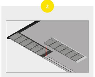
READYSLATE's modular design makes installation extremely simple. Aligning the modules is even easier as you overlap the second module over the remaining waterproof sheet of the previous module.
