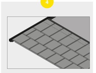
Repeat, easily adapting modules to any roof element, to complete your own waterproof, resistant and eco-friendly natural slate roof.
