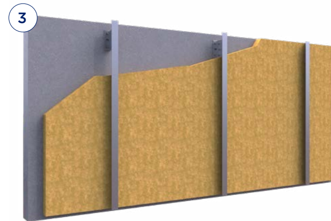
Fixing the "L" shaped profiles
